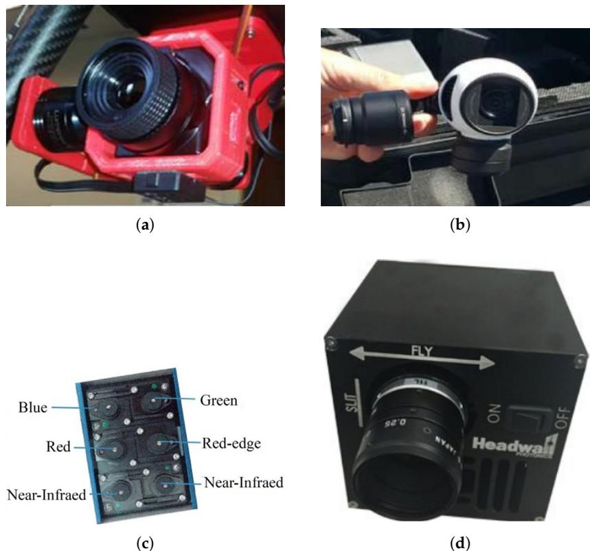
**Figure 2.** Examples of sensors used by UAVs for PA: (a) thermal sensor [103]; (b) RGB sensor [59]; (c) multispectral sensor [26]; and (d) hyperspectral sensor [88].
