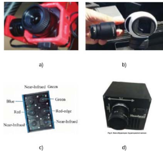
Fig. 1. Sensors used on UAVs for Precision Agriculture. a) Thermal sensor [27] b) RGB sensor [28] c) Multispectral sensor [29] d) Hyperspectral sensor [30]
