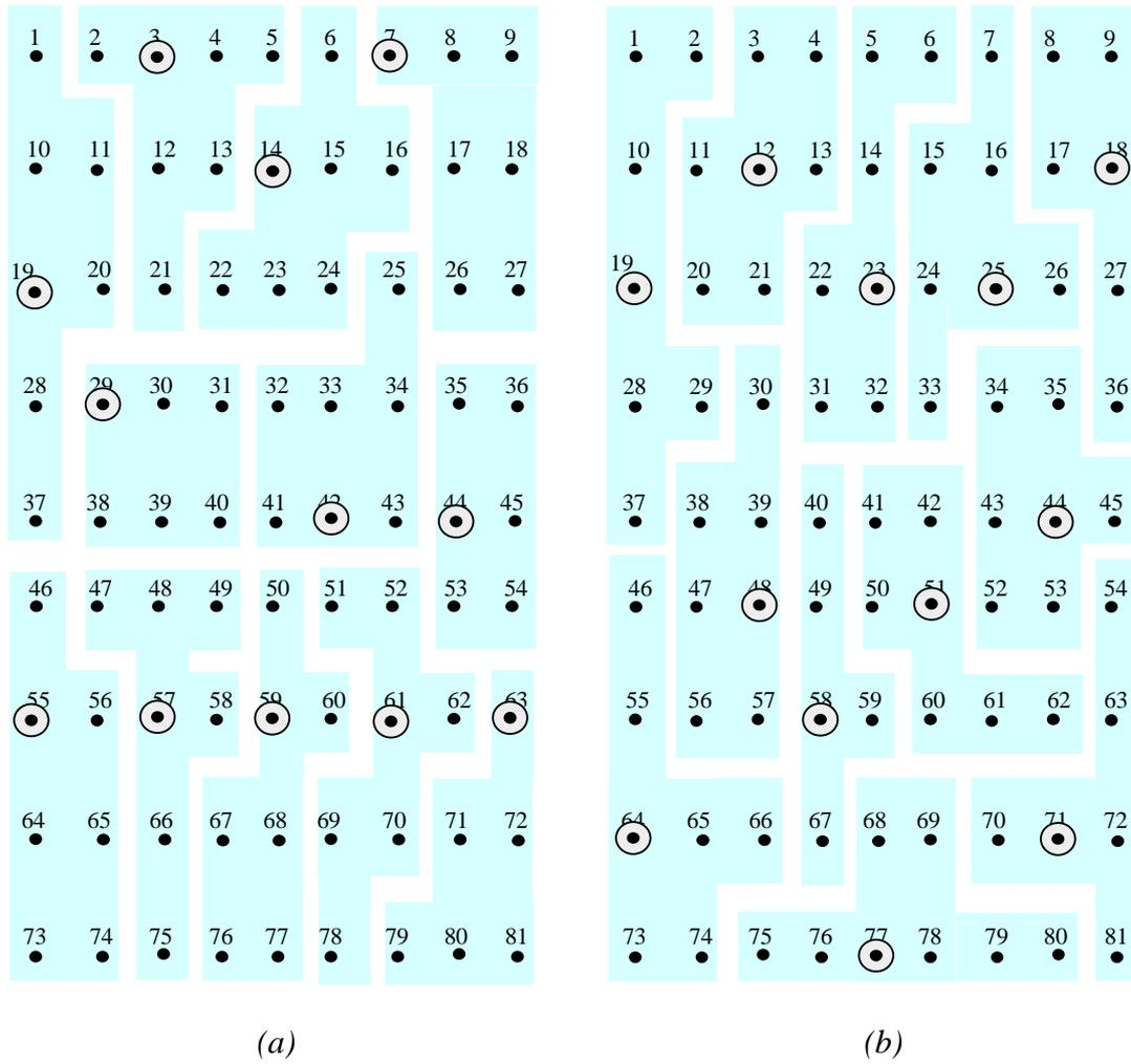
Figure 12(a)-(b). Allocation of BTSs to CSSs, when the BTS structure is the one depicted in Figure 7(b) and the CSS capacity is taken equal to 450000 cps and (a) the greedy algorithm is applied and (b) the simulated annealing algorithm is applied
