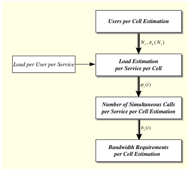
Figure 6. Bandwidth estimation process
