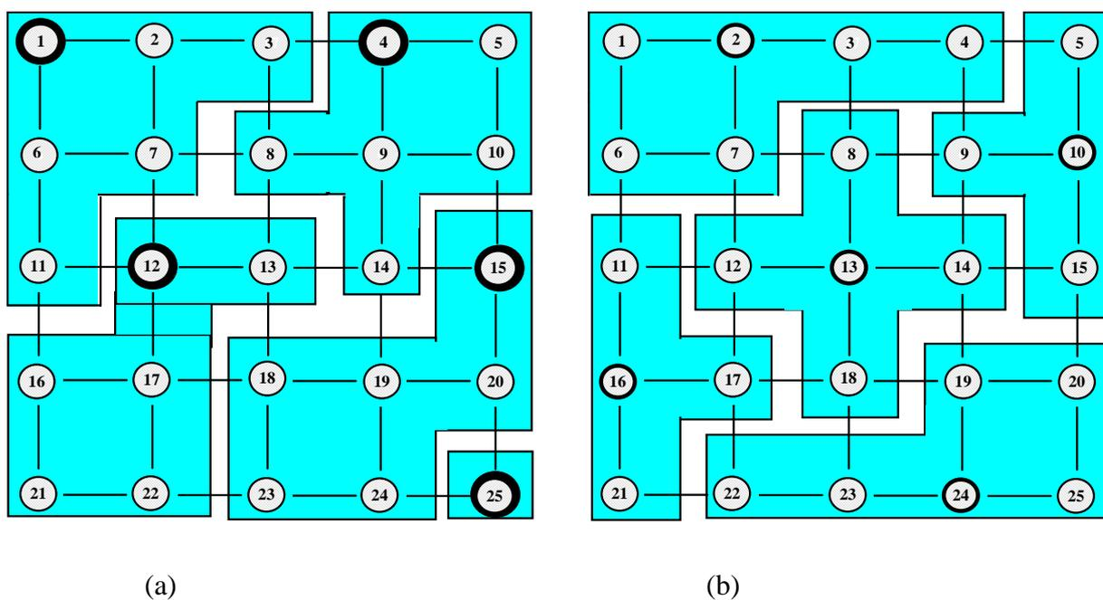
Figure 8(a)-(b). Allocation of BTSs to CSSs, when the BTS structure is the one depicted in Figure 7(a) and the CSS capacity is taken equal to 350000 cps and (a) the greedy algorithm is applied and (b) the simulated annealing algorithm is applied
