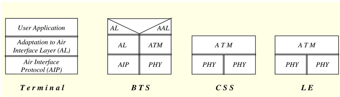
Figure 4. Protocol stacks supporting the ATM-based interconnecting network
