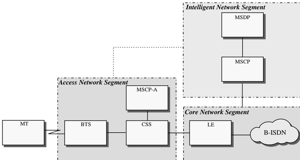
Figure 1. UMTS system architecture - Reference configuration
