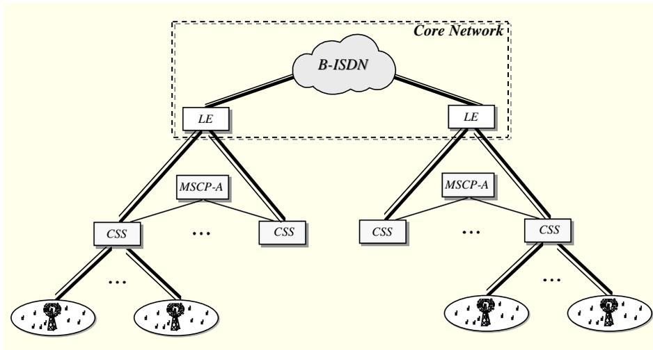
Figure 3. Architecture of the interconnecting network of the access segment of future cellular networks
