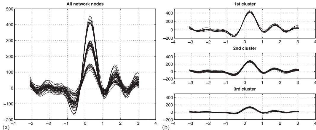
Figure 4. Andrews' curves: each curve depicts a node based on  $w=10$  channels: (a) nodes before clustering and (b) nodes after clustering.
