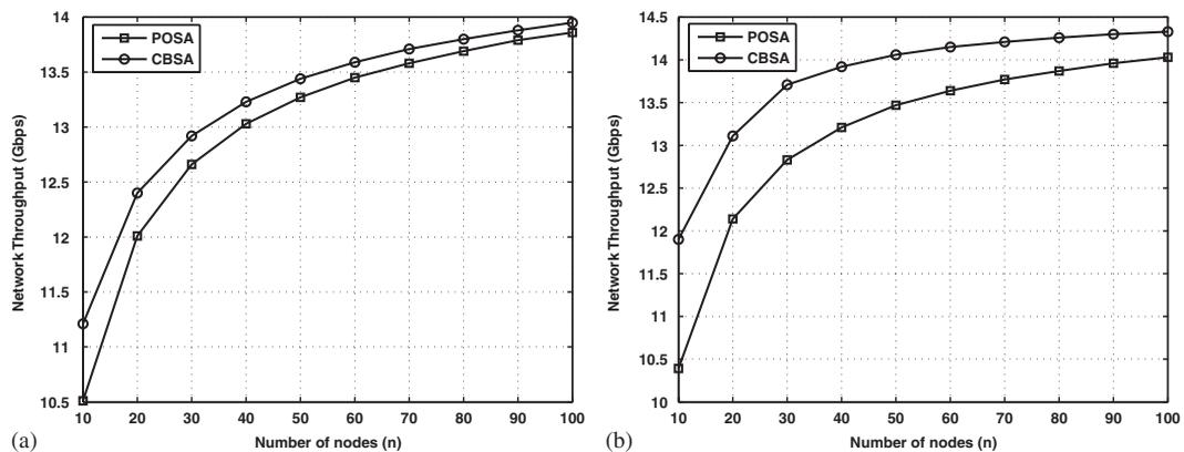
Figure 6. Network throughput as a function of the number of nodes for  $w = 5$  channels, traffic load  $k = \lfloor (n * w) / 5 \rfloor$  and  $\text{noc} = 6$  clusters: (a) uniform model and (b) asymmetric model.
