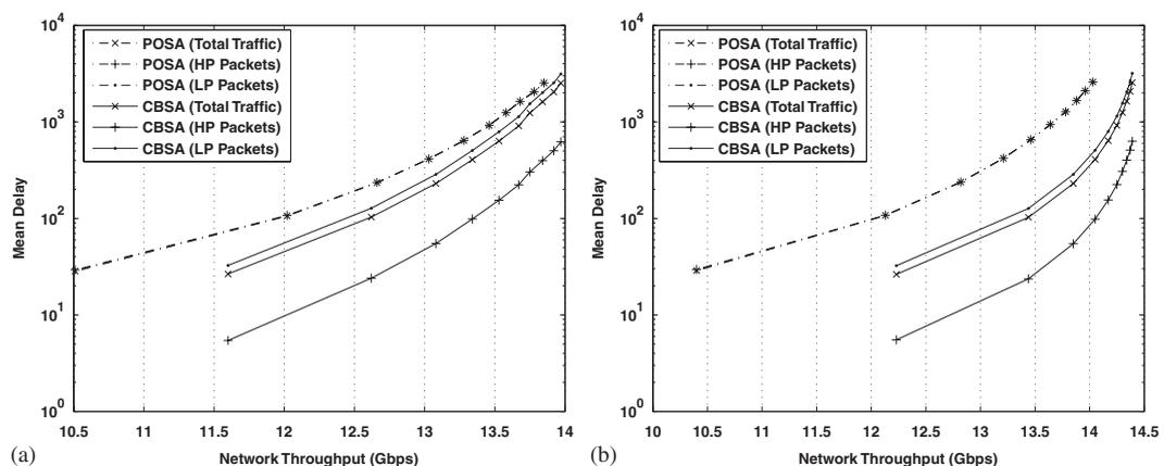
Figure 11. Mean packet delay of total traffic, high-priority and low-priority packets as a function of the network throughput: (a) uniform model and (b) asymmetric model.
