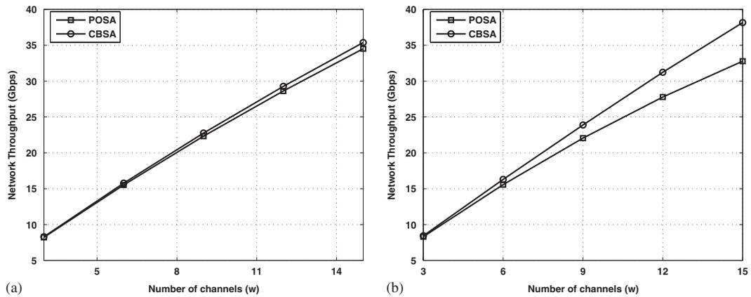
Figure 8. Network throughput as a function of the number of channels for  $n=40$  nodes, traffic load  $k=10$  and  $noc=6$  clusters: (a) uniform model and (b) asymmetric model.
