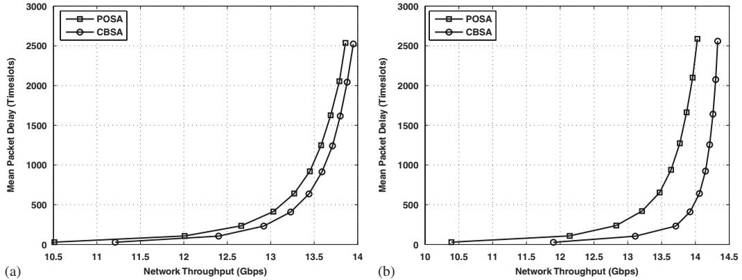
Figure 7. Mean packet delay as a function of the network throughput for  $w=5$  channels, traffic load  $k = \lfloor (n * w) / 5 \rfloor$  and  $noc=6$  clusters: (a) uniform model and (b) asymmetric model.
