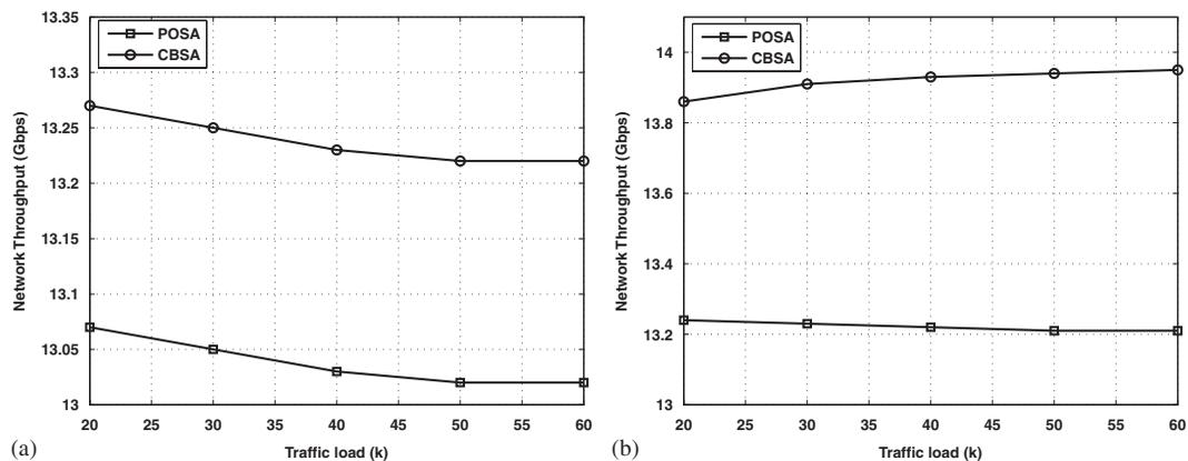
Figure 9. Network throughput as a function of the traffic load for  $n=40$  nodes,  $w=5$  channels and  $\text{noc}=6$  clusters: (a) uniform model and (b) asymmetric model.
