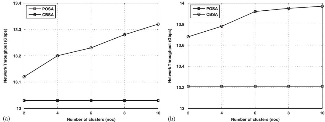
Figure 10. Network throughput as a function of the number of clusters for  $n=40$  nodes,  $w=5$  channels and traffic load  $k = \lfloor (n*w)/5 \rfloor$ : (a) uniform model and (b) asymmetric model.
