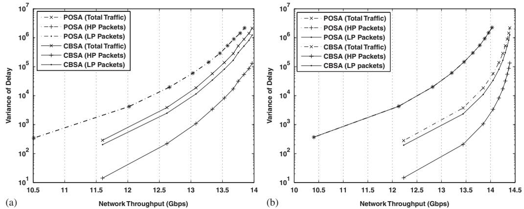
Figure 12. Variance of delay of total traffic, high-priority and low-priority packets as a function of the network throughput: (a) uniform model and (b) asymmetric model.
