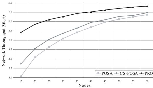
Fig. 2. Network throughput with eight channels.
