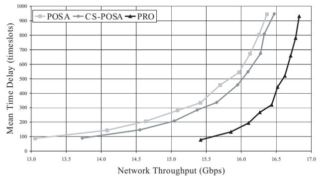
Fig. 4. Network throughput vs. mean time delay with eight channels.
