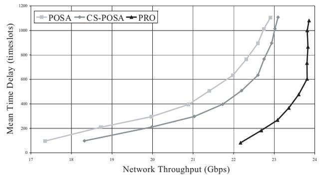
Fig. 5. Network throughput vs. mean time delay with 12 channels.
