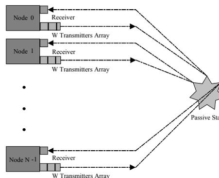
Figure 1. The network consists of N nodes and W channels, connected via a passive coupler.
