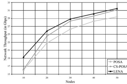
Figure 11. Network Throughput for 16 channels.
