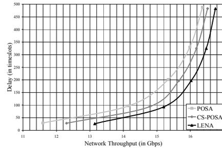
Figure 12. Throughput vs. Delay for 8 channels.
