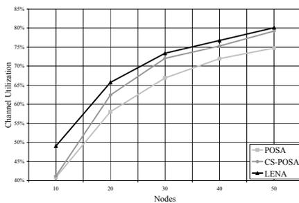
Figure 9. Channel utilization for 16 channels.
