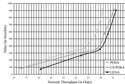
Figure 13. Throughput vs. delay for 16 channels.
