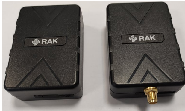
Fig. 4. RAK7200 SMA to UFL modification
